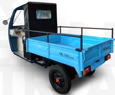
E Cart with Carriage Box & Hydraulic Tipping Mechanism
